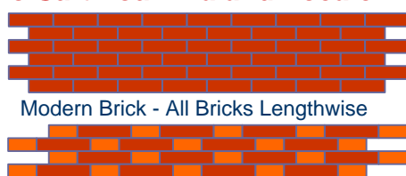
Flemish Bond - Alternate Brick On-End
